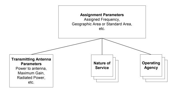
It is to be noted, that this structure provides only for a single set of transmitting antenna parameters, in line with the concept of typical station (No. 11.17 of the RR).
