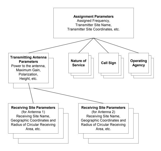
As shown in the above diagram, this notice has two sets of transmitting antenna parameters ("antennas"), each with its own set of three receiving sites. In fact, there is *no* limit concerning the number of "antennas" for one notice, and *no* limit concerning the number of receiving sites per antenna. Note, however, that the precise parameters for the assignment, the antenna, and the receiving site vary according to the Notice Type; the fields shown above are merely examples.
