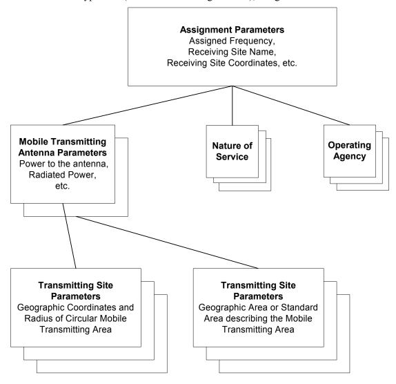
As shown in the above diagram, this notice has two sets of transmitting antenna parameters ("antennas"), each with its own set of three transmitting sites. In fact, there is *no* limit concerning the number of "antennas" for one notice, and *no* limit concerning the number of transmitting sites per antenna.
